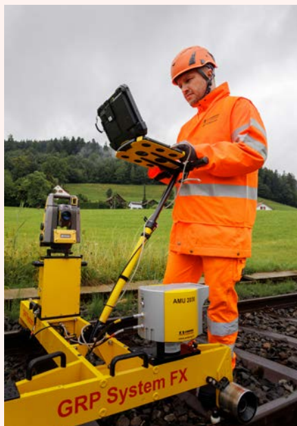
▲ Capturing and analysing track data with the Topcon and Amberg rail surveying system.
