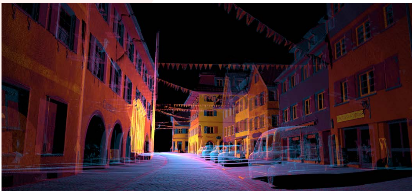
▲ A Lidar point cloud.
