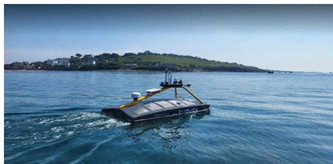
▲ An XOcean USV departs on an autonomous bathymetric survey mission in the UK Atlantic. (Image courtesy: UKHO)
