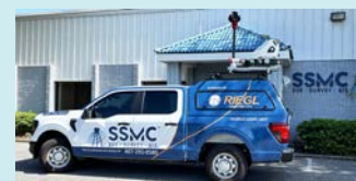
▲ Fully equipped and field-ready: SSMC’s newest mobile Lidar vehicle with the VMX-2HA mounted. (Image courtesy: RIEGL, SSMC)
