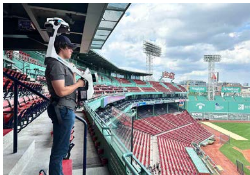
▲ The technology's reach now extends far beyond factories and construction sites. US-based BIMstream has used the NavVis VLX to map a baseball stadium, for instance. (Image courtesy: BIMstream / NavVis)
