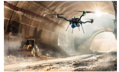
▲ Hovermap can be mounted on a drone (as shown here surveying a tunnel) or a robot, or can easily be switched to handheld, backpack, vehicle or pole-mounted scanning. (Image courtesy: Emesent)
